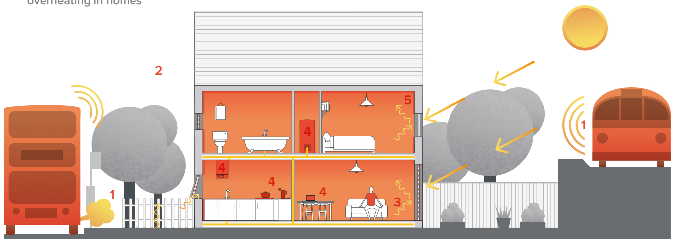
Figure 7. Illustration adapted with kind permission from 'Understanding Overheating – Where to start' (NHBC Foundation NF44, 2012) showing some of the causes and cumulative effects of overheating in homes
